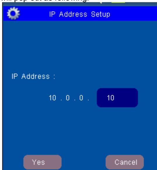
**Figure 10: Window for Ethernet IP Address Setup**
